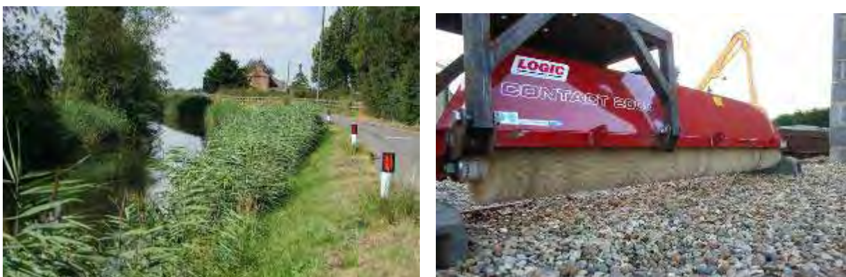
Left. Reed growth on Well Creek that can extend up the bank and become a traffic hazard. Right. A brush type weed-wiper that has been adapted to replace a flail mower head as a potential method to provide more targeted delivery of herbicide close to water.
